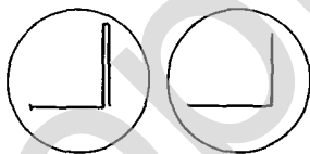
1 1/4" Standing Seam With Right Angle Flange Up to 1 1/2" available Both standing seam and right angle flange are formed with same roll set
