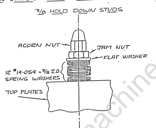
WHEN INSTALLING TIGHTEN JAM NUT UNTIL SPRING WASHERS FREE FLAT THEN BACK OFF ONE TURN AND TIGHTEN ACOEM NUT.
