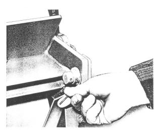
An eccentric pin at the rear of the beam allows the bending edge to be set from 0 to 1/8" back from the edge of the bed. This provides clearance for the material, and a reasonable radius, when the apron is lifted to make a bend. Normal clearance is a space of 1 1/2 to 2 times thickness of material between apron and bending edge, when the apron is at 90 degrees.
